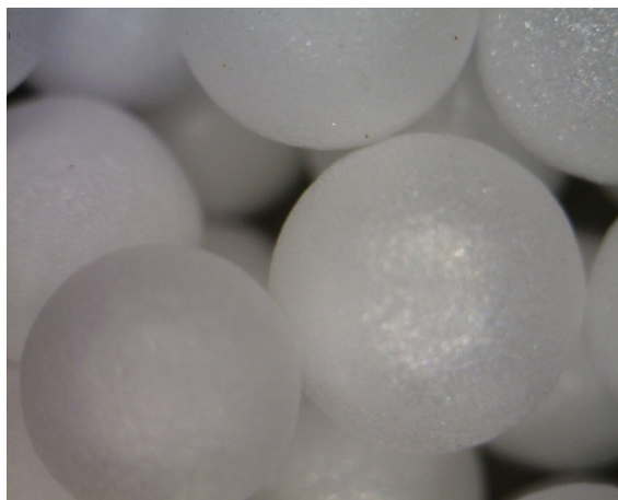
Figure 4: EPS granules recorded by microscope (magnified 50×).
